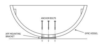
NOTE: Drainage MUST be provided in the bottom of each bowl.
