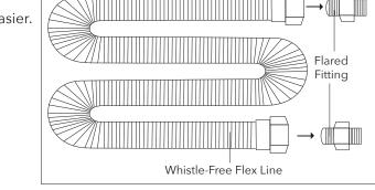
Apply thread sealant here 1/2" x 3/4" Reducing
