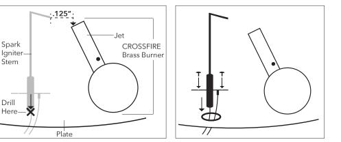
If the distance to the jet is greater than .125", you can adjust the position by **gently** bending the spark ignitor by the stem. Bending too far can result in breakage. Do not flex at the existing bend, this can result in breakage. If the spark ignitor is too far away or too close to the jet, you will not get a strong enough spark to light the burner.
