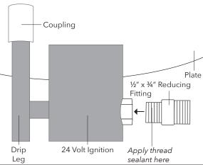
**3A. CONNECT TO COUPLING** (FK2) Do not use 1/2" x 3/4" reducer fitting with this install. Connect ¾" x 3" Nipple to Gas Valve.
