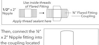
on the bottom of the aluminum plate. Tighten.
