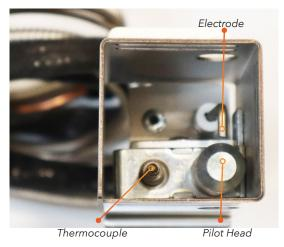
Photo 3b: Top-Down View of Pilot Assembly
