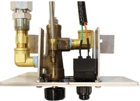
5.2 The pilot tube connects directly above the thermocouple. Thread the pilot tube into the brass fitting integrated into the valve body that is directly above the thermocouple connection. [See Photo 14]. Tighten with a
