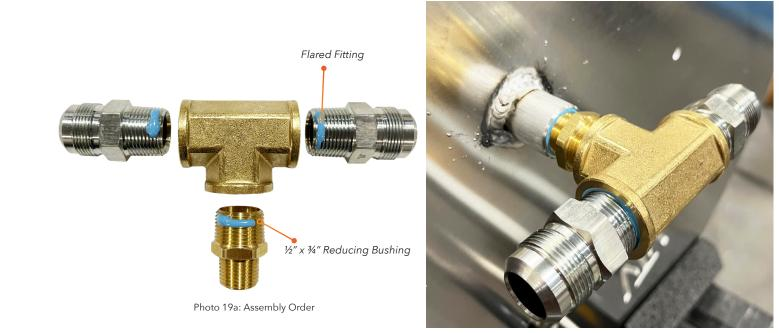
6.4 WITHOUT ANY THREAD SEALANT take the other end of the flex line attached to the valve assembly from Step 4 and attach the female flared end to the male flared end that is attached to the plate from Step 6.3. [See Photo
