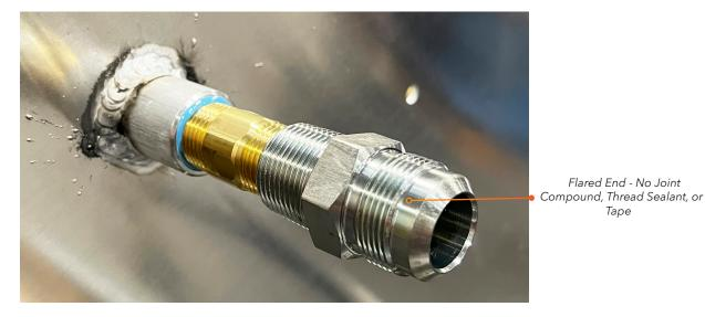
Photo 17: Attaching the Male Flare Hose Adapter
