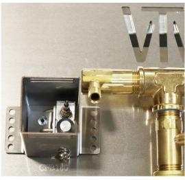
Photo 4a: Thermocouple Positioning
