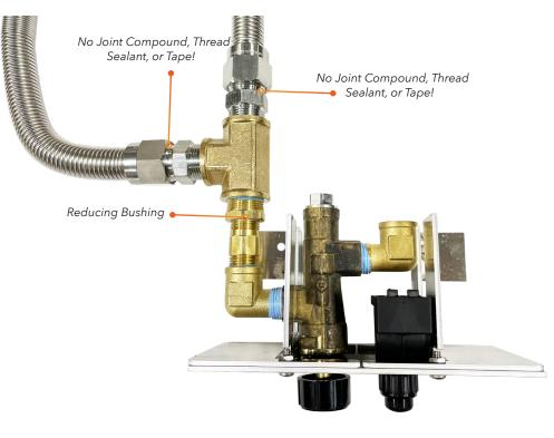
Photo 12: Final Assembly with Flex Lines Connected
