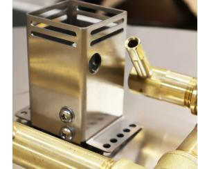
Photo 4b: Pilot Hood Circular Opening Positioning
