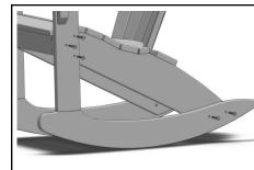
Place Seat Assembly on it's side, using a flat clean surface. Place Rocker Assembly with mounted support over seat assembly, while making sure the mounted support is facing outward. Insert (5) 75mm connector bolts through the predrilled holes in the Rocker Assembly and align this with the pre-drilled holes in the seat assembly. Finger tighten flat washer, lock washer, and nut on each bolt. Do not fully tighten at this time. Flip the assembly over and repeat process for opposite Leg.
