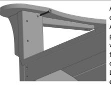
Arms should be installed with curve cutout on the inside of the chair. Place Arm on top of Front Leg. Align pre-drilled hole in the Underarm support with the pre-drilled hole located at the top of the Front Leg. Install a 75mm connector bolt, starting from the Front Leg through the Underarm. Finger tighten flat washer, lock washer and nut. Do not fully tighten at this time. Repeat process for opposite Arm.
