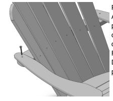
Place Upper Yoke of the Back Assembly underneath arms, aligning pre-drilled holes. Install (1) 60mm connector bolt through pre-drilled hole of the Arm and through Upper Yoke. Finger tighten flat washer and lock nut. Do not fully tighten at this time. Repeat process for opposite Arm.
