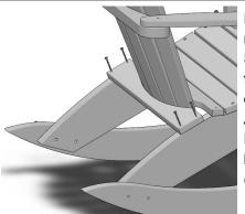
Place Back Assembly on top of mounting surface of Rear Legs (Part of Seat Assembly). Push Back Assembly forward until it meets the last Seat Slat of the Seat Assembly. Hold Back Assembly in place and install (4) 1-3/4" Phillips Head Screws into pre-drilled holes on each side of the Lower Yoke (No pre-drilled holes on Rear Legs).
